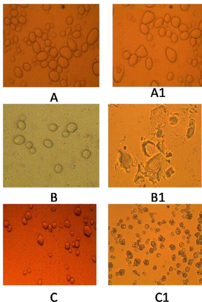
**Figure 1.** Native and hydrolyzed starch under optical microscope at 40X magnification: (A) Native potato; (A1) Hydrolyzed potato; (B) Native corn; (B1) Hydrolyzed potato; (C) Native Commercial corn starch; (C1) Hydrolyzed commercial corn starch
