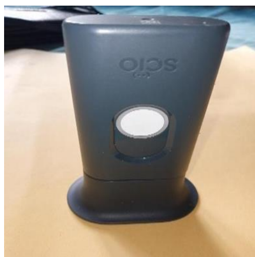
Figure 1. (a) Process flowchart of production of Komal Chaul ; (b) NIR Sensor with sample holder
