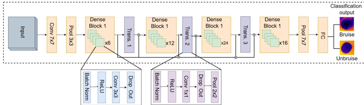
**Figure 4.** A simple representation of the DenseNet121 model
