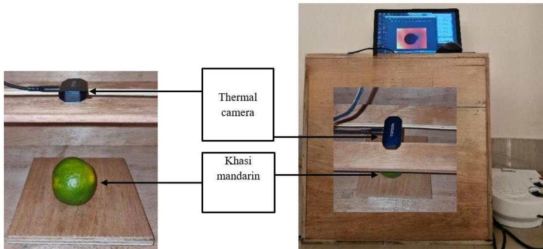
**Figure 2.** Experimental setup for thermal imaging and image processing unit
